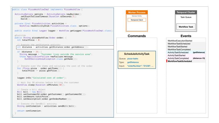
The cluster then adds another Workflow Task to drive the Workflow Execution forward.
