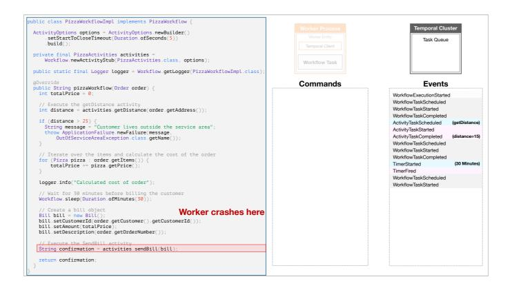
Workers are external to the cluster and operate with autonomy. They long-poll the Task Queue, but only when seeking work to perform. They retrieve tasks from the queue, rather than being assigned tasks directly by the cluster.
