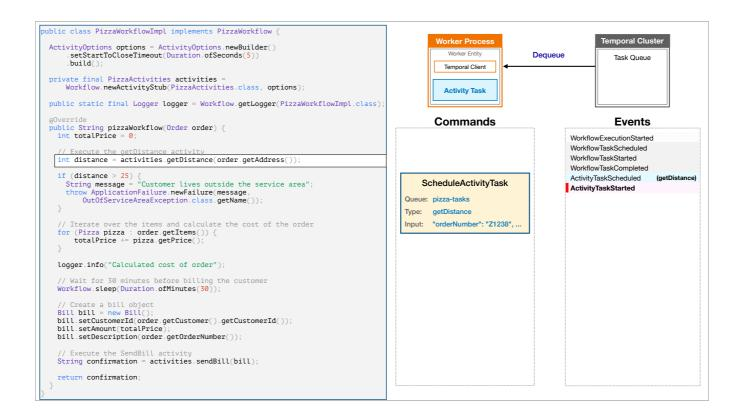
The cluster logs an Event to signify that the Worker has started the Activity Task. I've shown this in pink to indicate that it's the indirect result of the Command.
