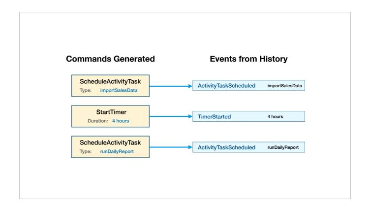
If a specific Command results in a specific type of Event, then it follows that the reverse is also true. In other words, given one of these Events, you can determine which Command led to that Event.
