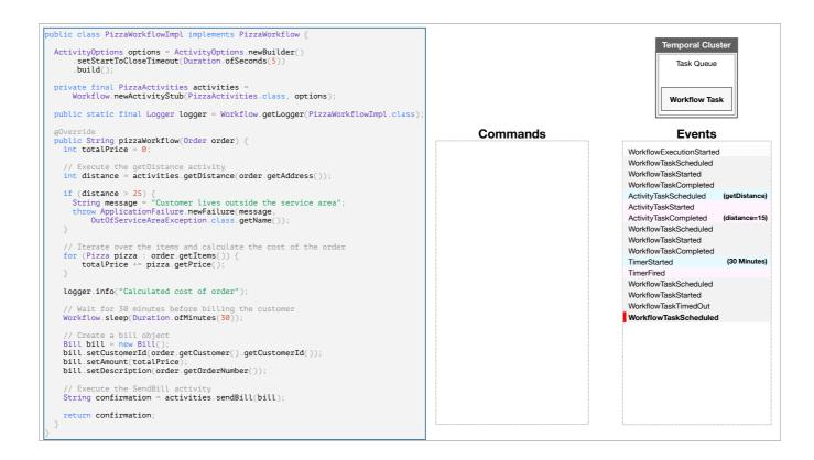
Therefore, if the Worker failed to complete this Workflow Task within that time, the cluster assumes that the Worker has gone down, and will schedule a new Workflow Task.
