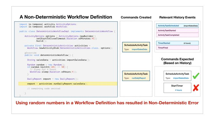
Since the Workflow Definition produced a different sequence of Commands during replay than it did prior to the crash, the Worker is unable to restore the previous state, so the use of random numbers in the Workflow code has resulted in a non-deterministic error.
