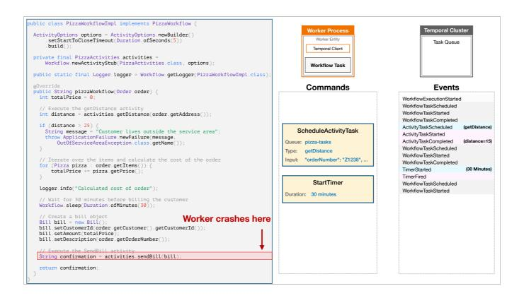
However, let's suppose that the Worker happens to crash right here. How does Temporal recover the state of the Workflow?
