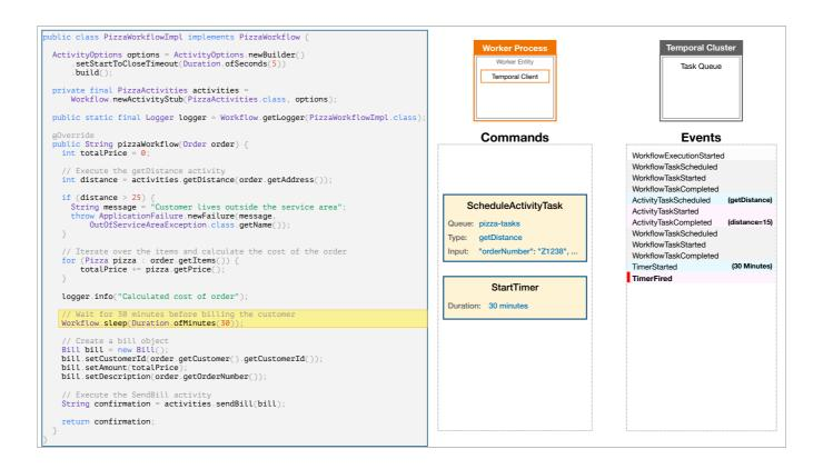
After 30 minutes has elapsed, the Timer fires, and the cluster logs a TimerFired Event. How does the Worker know that it can continue running the Workflow code now?
