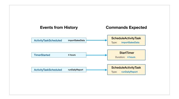
The Worker uses this logic to evaluate the Event History during replay and validate that it can reliably recover the Workflow Execution.
